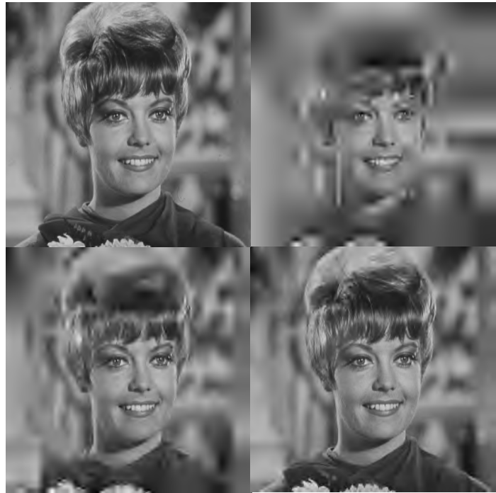
Fig. 4 Foveated rate scalable compression results of “Zelda” image (Upper-left, 512×512, 8bits/pixel) using the weighting model in Fig. 3(b). The compression ratios are 1024:1 (Upper-right), 256:1 (Lower-left) and 32:1 (Lower-right), respectively.
