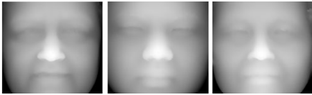
Fig. 10 The sub-regions of the facial range images that were employed for the eigensurfaces and fishersurfaces 3D face recognition algorithms
