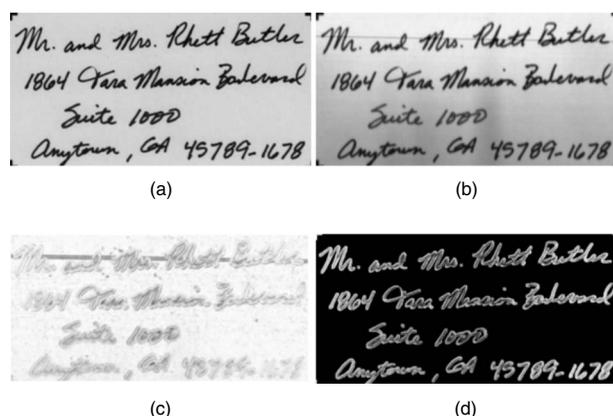
**Fig. 6** Evaluating the quality of handwritten text: (a) 600-dpi scan of the handwritten test target, (b) image of the handwritten text as scanned by a LSC, and (c) SSIM map between the 600-dpi and LSC image. Bright regions in the map indicate good quality, while dark regions indicate poor quality. (d) Masked SSIM map. SSIM index is computed only around the text areas.
