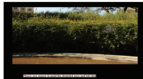
Fig. 4 : Image with local white noise distortion. The boundary was blended using a Gaussian blending window. When the image was presented, the subject was requested to point out the distortion by clicking the mouse cursor on the distortion.
