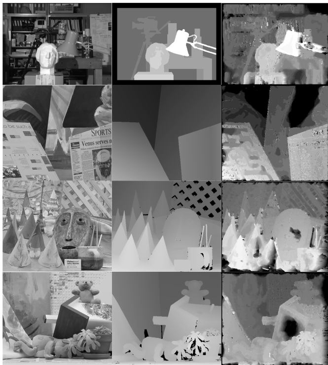
Fig. 19. Performance of the proposed stereo model on Middlebury stereo pairs. First row: Tsukuba ( B = 0.31 ), Second row: Venus ( B = 0.35 ), Third row: Cones ( B = 0.39 ), Fourth row: Teddy ( B = 0.40 ). Column 1: left image, column 2: ground truth disparity, column 3: estimated disparity.
