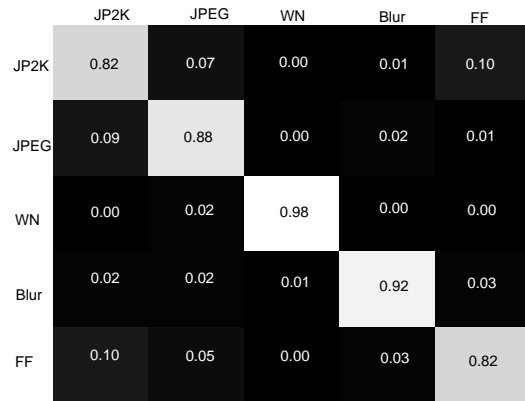
Fig. 10. Mean confusion matrix for classifier across 1000 trials: which row (distortion) is confused as which column (distortion). Higher number indicates greater confusion.
