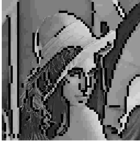
Fig. 3. The result of edge detection in the image Lena JPEG-coded at 0.217 bpp (the threshold T = 120 ). The detected edge blocks are marked as black blocks .
