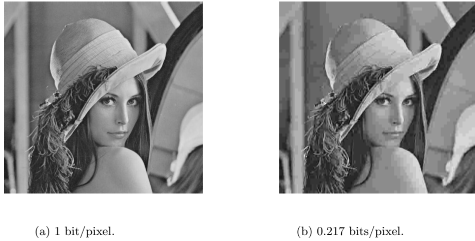
Fig. 1. Blocking effects in the image Lena JPEG-coded at different bit-rates.
