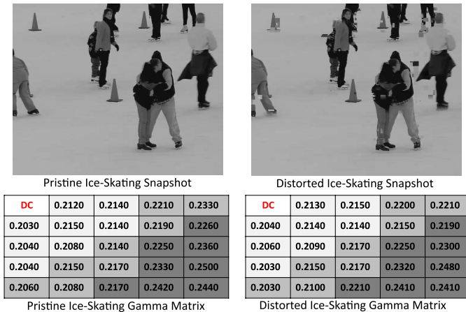
Fig. 11. Snapshots of the pristine and distorted Ice-Skating sequence, along with the computed \gamma matrices from corresponding frame-difference DCT coefficients. Notice how the \gamma values differ between the pristine and distorted sequences.
